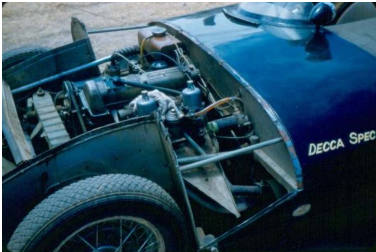
Decca Mk2 Climax, Collingrove Hillclimb circa 1957. Coventry Climax 1097cc FWA SOHC, 2 valve, twin SU carburetor engine to 'Stage 2' tune giving circa 83 bhp @ 6800 rpm (K Drage)
