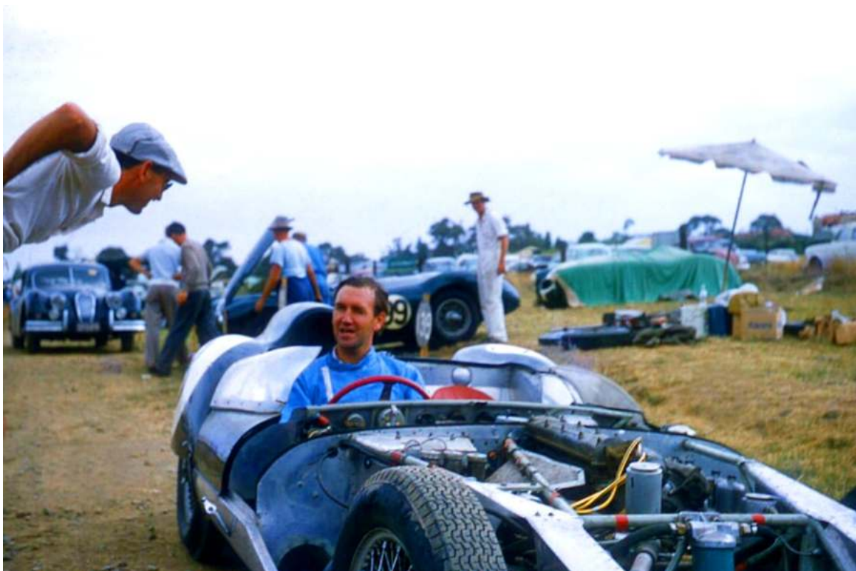
Derek looking pretty happy with the car '608/626' in the Gnoo Blas paddock February 1960. Is that Jack Myers he is speaking to? Jolly's tow car XK140 behind, car with bonnet up is Tom Sulman's Aston DB3S. You can see the slight canting of the FPF engine, cars spaceframe chassis and cross bracing in the engine bay referred to in the text (Kelsey)
